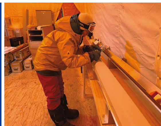
Determining the depth of an ice core drilled at Dome Fuji Station II. The ice core is in the right foreground of the image.
